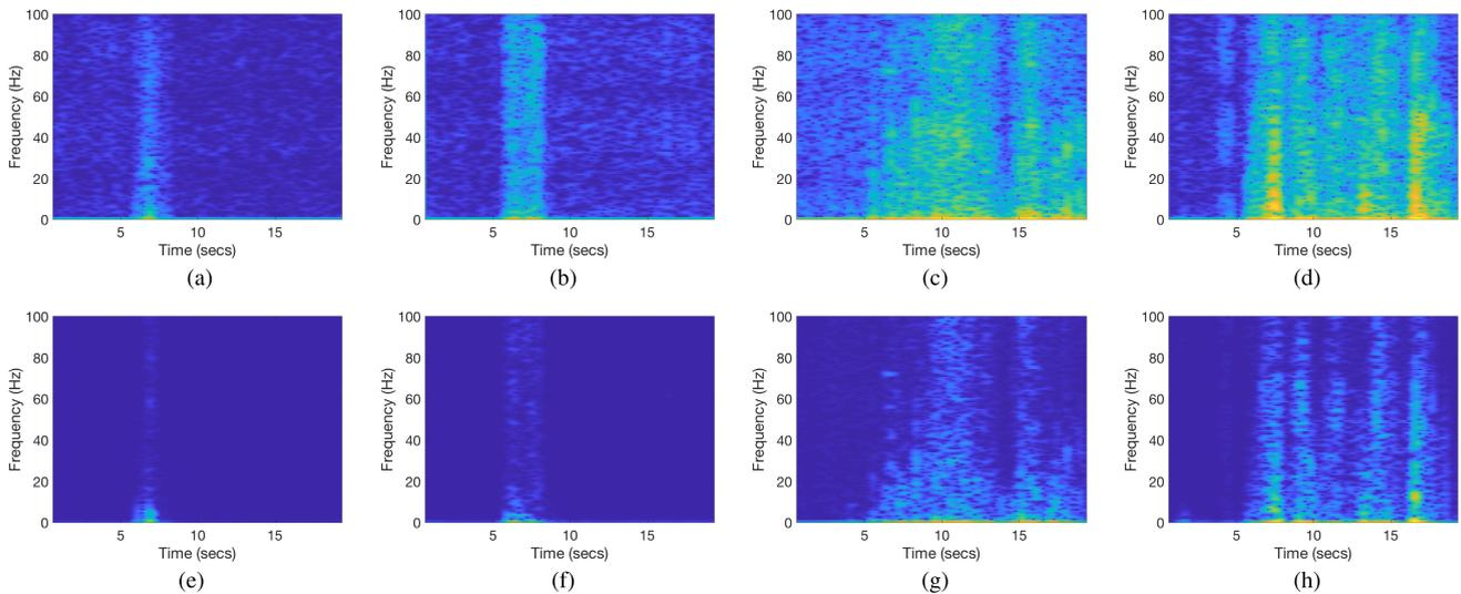
**FIGURE 8.** Spectrograms for 4 activities (falling, lying down, walking, and running) using two subspace update variants: batch and stochastic. It is readily that stochastic has a filtering effect on the time-frequency localization of pairwise differential unitarity subspace tracking metric. (a) Falling – batch. (b) Lying down – batch. (c) Walking – batch. (d) Running – batch. (e) Falling – stochastic. (f) Lying down – stochastic. (g) Walking – stochastic. (h) Running – stochastic.
