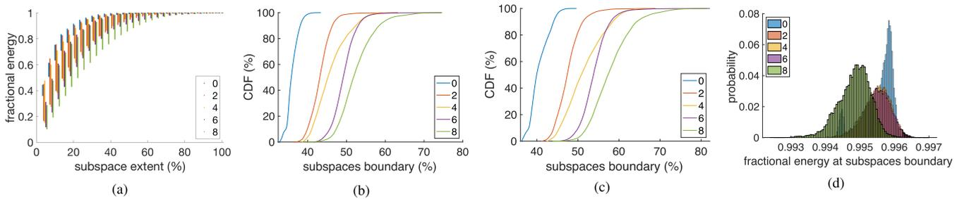
**FIGURE 3.** Characterizing signal and noise subspaces through an MSE search procedure for 5 uncontrolled human movement scenarios. The numbers in legend 0, 2, 4, 6, and 8 denote how many moving people are present. (a) Fractional energy  $E_s$  evaluated across the signal dimensionality. (b) MSE-based subspace boundary at  $-6$  dB reconstruction objective. (c) MSE-based subspace boundary at  $-12$  dB reconstruction objective. (d) Fractional energy at subspace boundary.
